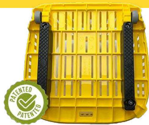
The basket rests securely on the ramp or escalator, preventing it from sliding down. Our new braking system consists of a couple of pieces bolted to the basket, which prevents the basket from slipping, as the wheels do not touch the ground and therefore the basket cannot slide.
